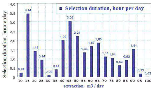
Figure 1. Results of the frequency analysis of the time series of water consumption.
