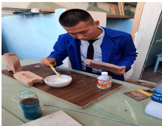
Fig. 5. External treatment with a silicon solution
