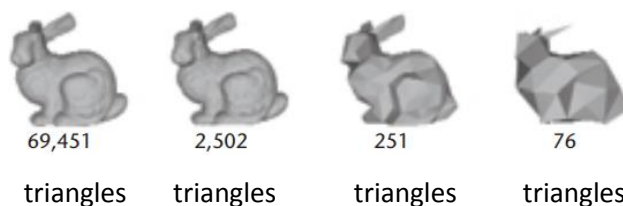
Fig. 7. Managing model complexity by varying the level of detail used for rendering small or distant objects. Polygonal simplification can create multiple levels of detail such as these.
