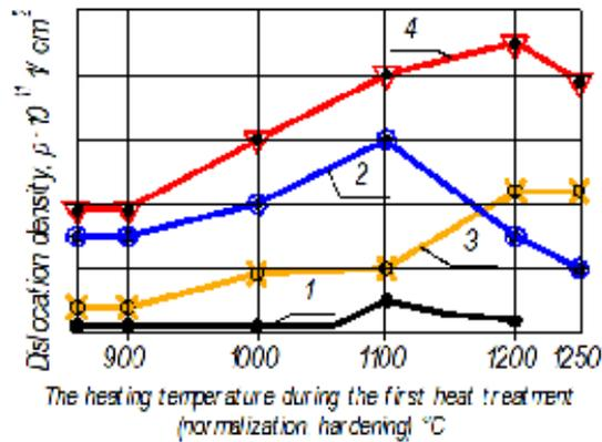
**Fig. 6.** The scheme of formation of the fine structure of steel after double phase recrystallization: 1 - initial normalization; 2 - during hardening with  $Ac_3$  (or  $Ac_1$ ) + 30 ÷ 50 °C; 3 - growth of lattice micro distortions due to secondary intragranular texture; 4 - the total effect of increasing dislocation density
