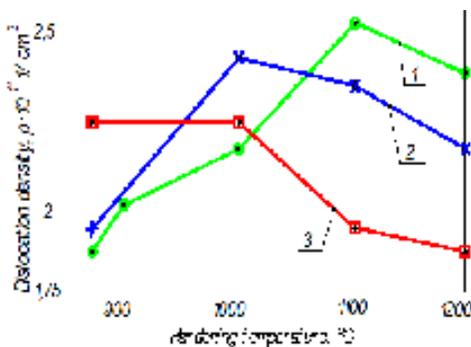
**Fig. 4.** The effect of temperature and heating time on the density of dislocations in hardened steel 45. Tempering during heating 200 °C. Holding time during heating: 1 - 20 minutes; 2 - 2 hours; 3 - 5 hours
