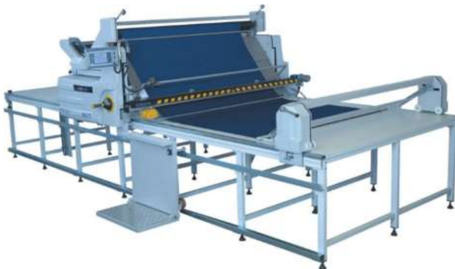
1.10-rasm. Og'irligi 350kg bo'lgan MJ1 Master Jeans markali rulon gazlamalarni avtomatik ravishda milknini to'g'rilab to'shash mashinasi
