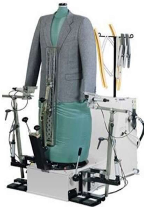
2.13-rasm. Yenglarni dazmollash uchun, Germaniyaning "TEST" firmasining ARAP pressi
