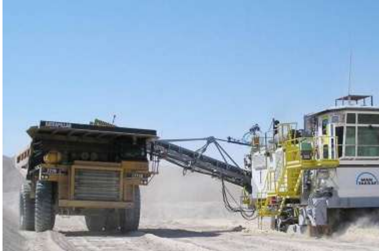
Fig. mining of ore by MTS-250 combine with loading into a SAT-777D dump truck
