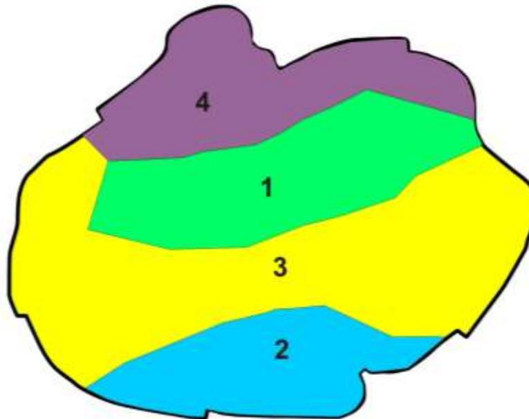
**Figure: 1.** Scheme of dividing the working area of the Muruntau open-pit mine into active and passive parts: 1 - non-working open-pit side; 2 - temporary rear sight; 3 - the main working area; 4 - "North Board".
